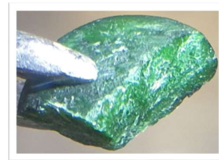
Solid ingots of frozen fuel of ~100% th. density
