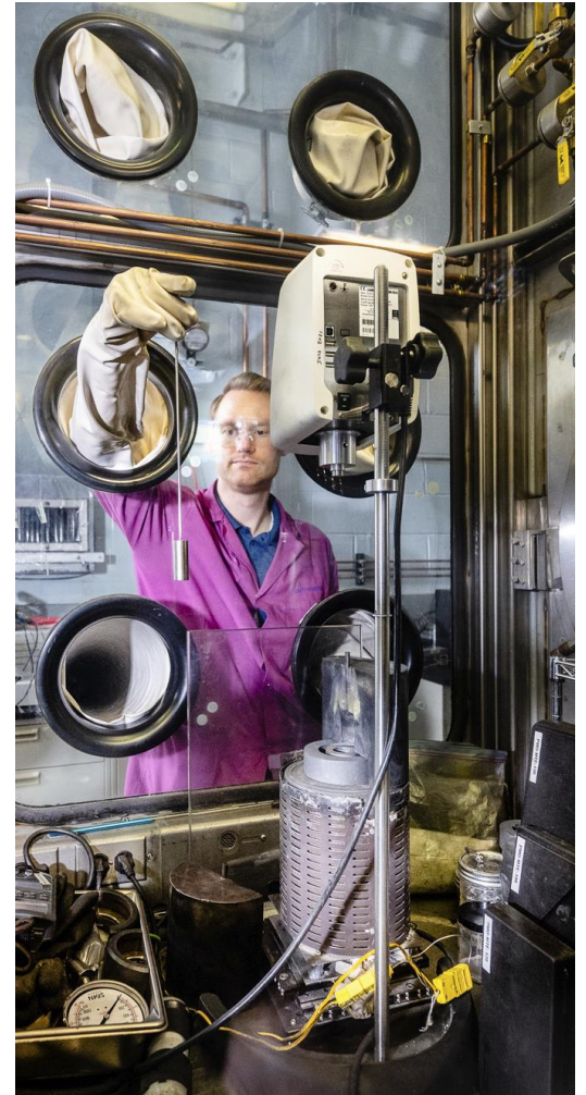
Rotational Viscometer Installed in a Glovebox for Measuring Molten Salt Viscosity
