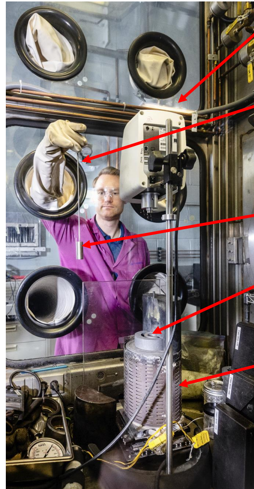
Viscometer apparatus installed in glovebox.
